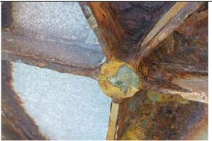
Dry/no grease caused the pin to freeze and eventually shear
